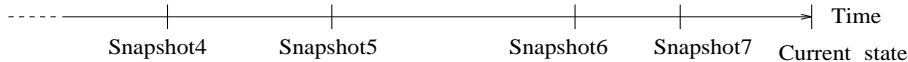
Figure 11.1: Snapshots represent consistent database states as of some time in the past.
